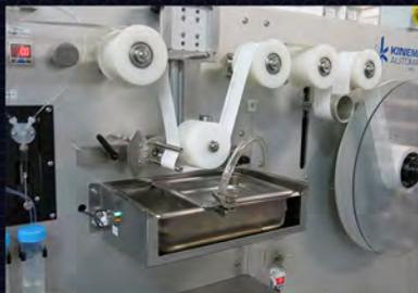
Optional dip tank with peristaltic pump
