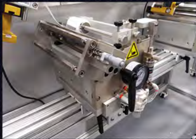
Lamination Station with Pneumatic Pressure
