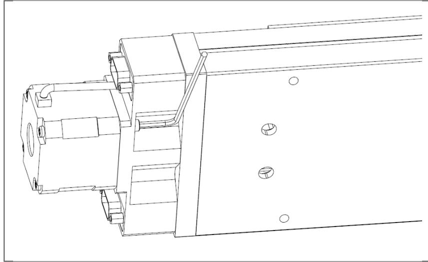
4) Fully tighten the coupling clamp screw.
