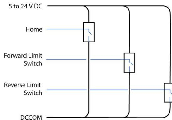
Figure 6-3: Equivalent Limit and Home circuit schematic
