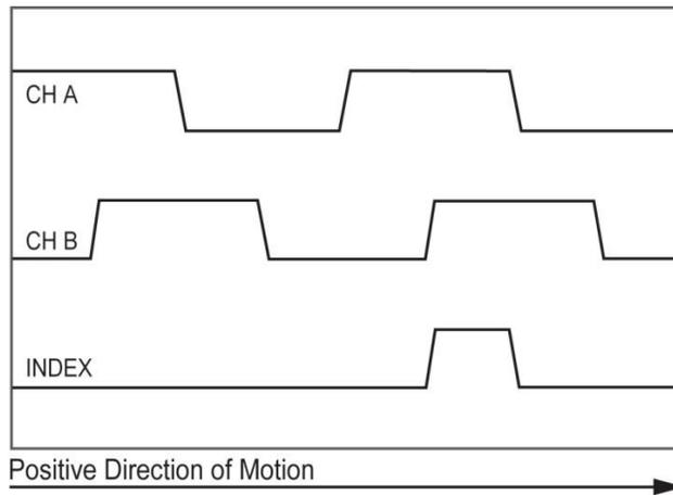
Figure 6-2: Timing diagram for the encoder signals
