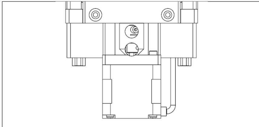
3) Mount the motor to the stage with four fasteners. A low clearance hex wrench may be required for tightening. Fully tighten all four fasteners.
