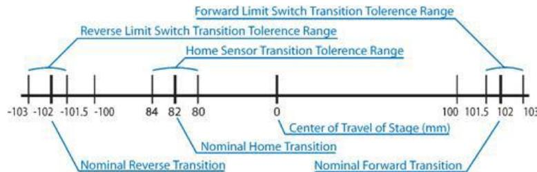
**Figure 6-4: Typical Sensor Transition Regions for Default Configuration (200mm travel example)**
